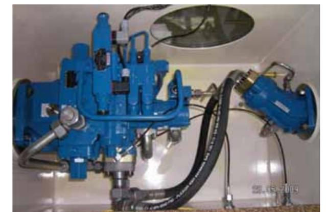
Figure 6: Closed loop system with variable pump
