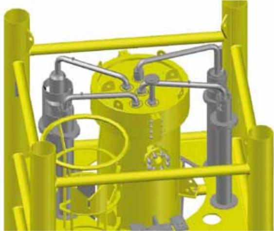
Figure 17: Subsea connector interfaces with piping
