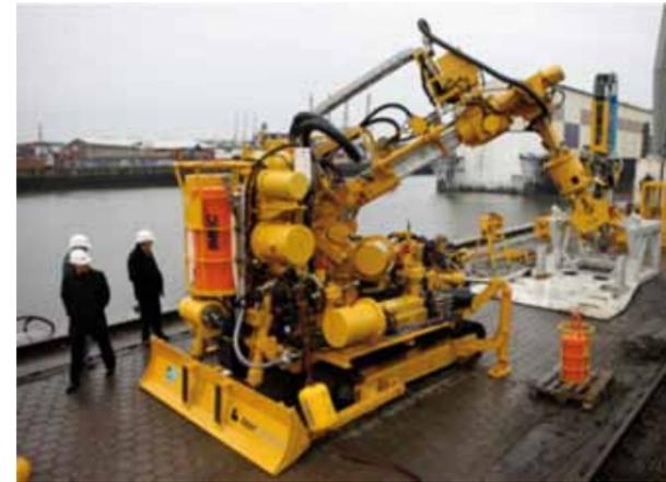
Figure 7: The IMPac-dCAS subsea boxes with the Seafloor Working Unit from Aker-Wirth during trials
