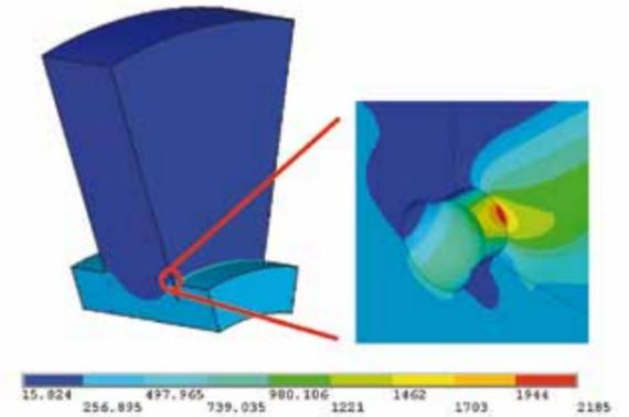
Figure 7: Stress model of a conveyor screw including a corrosion pit
