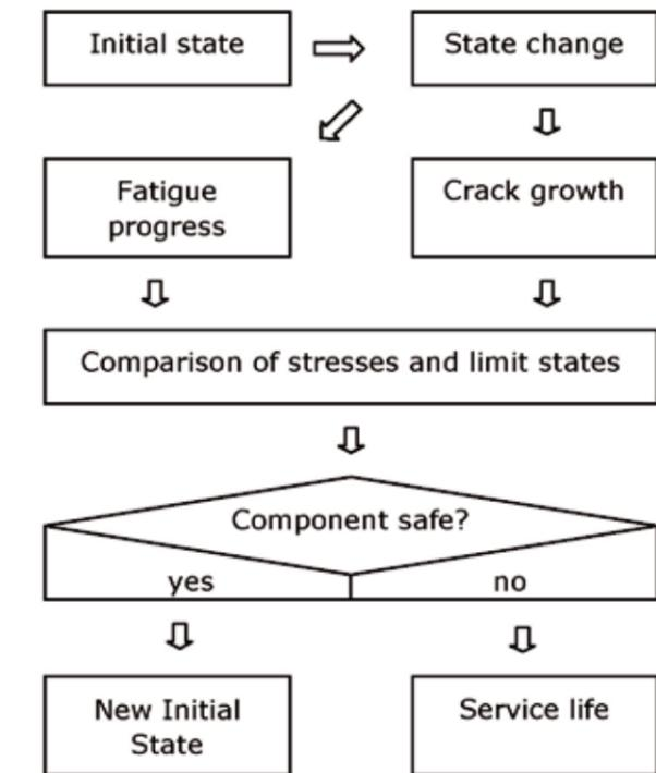
Figure 5: Graph of the new method for strength assessment incorporating corrosion and wear
