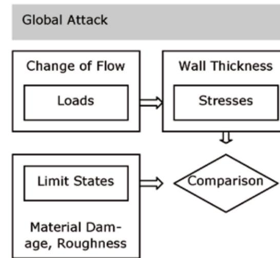
Figure 3: Effect of global attack on component strength
