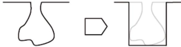
Figure. 12: Reduction of the real pit-shape to a simplified geometry in the static strength assessment
