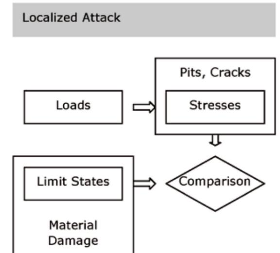
Figure 4: Effect of localized attack on component strength
