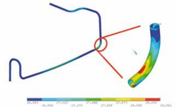
Figure 8: Stress model of a pipe bent
