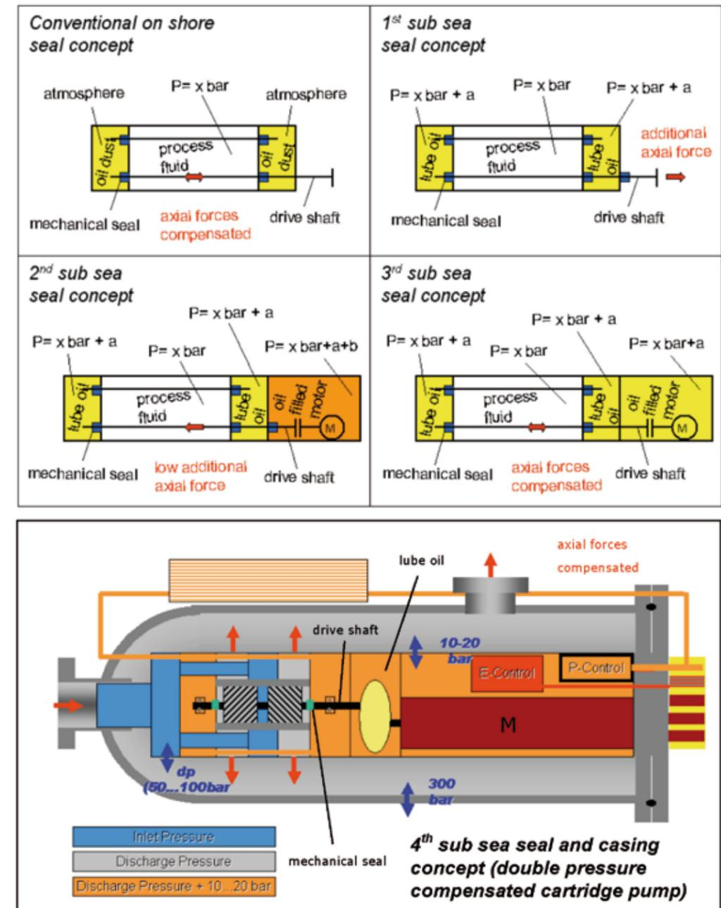
Figure 6: Concepts of mechanical seal arrangements for sub-sea pumps
