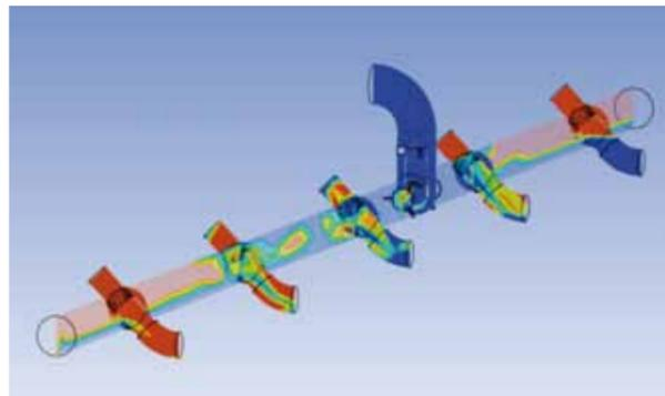
Figure 13: Flow simulation of conventional header
