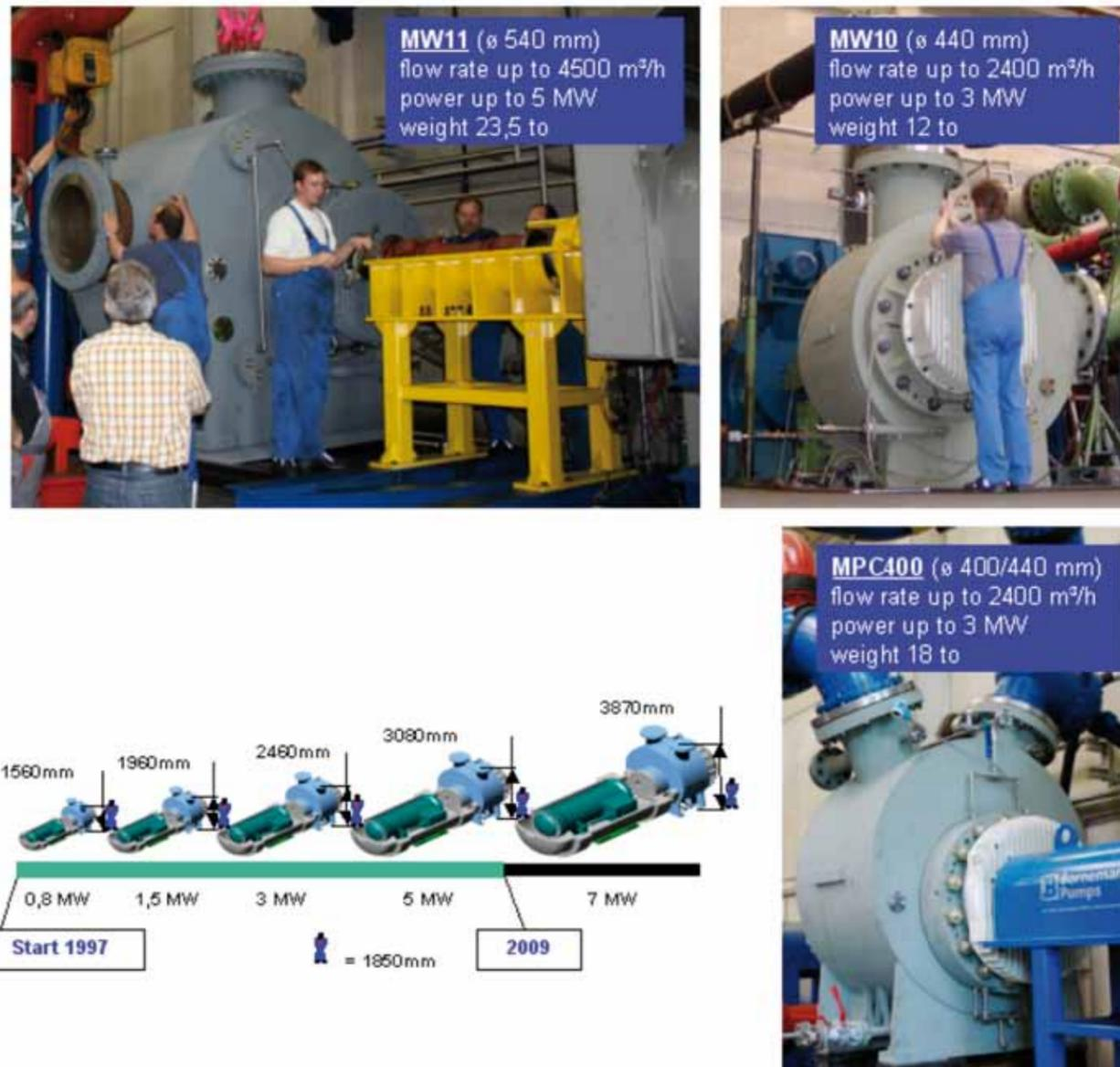
Figure 11: Multiphase pump sizes planned and realized
