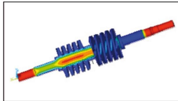
Figure 5: Heat distribution in engineered rotor
