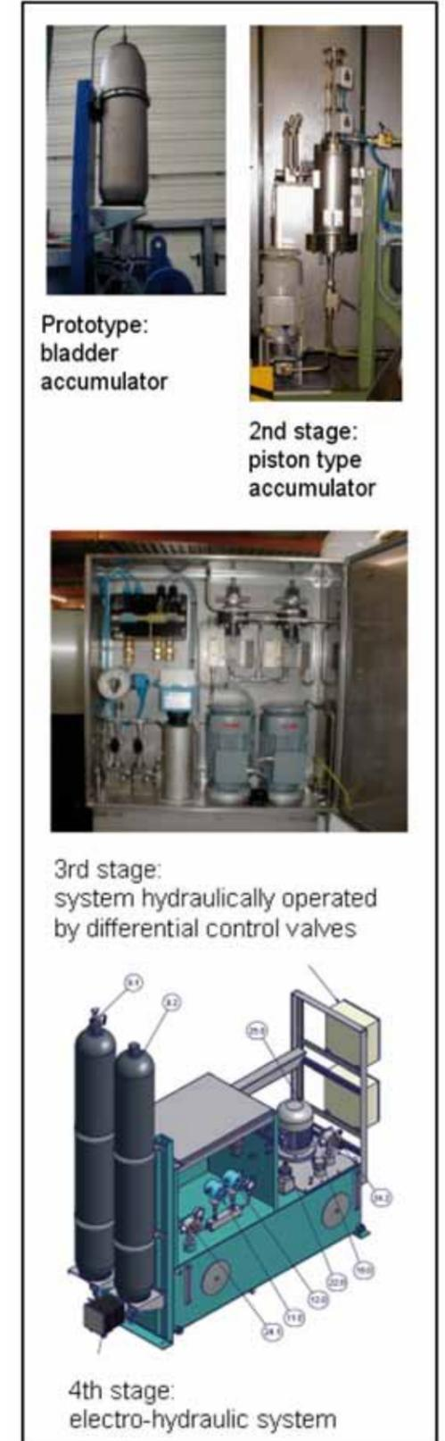
Figure 7: R&D stages of seal oil systems
