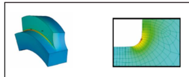
Figure 4: FE-Model of pump screw's tooth flank
