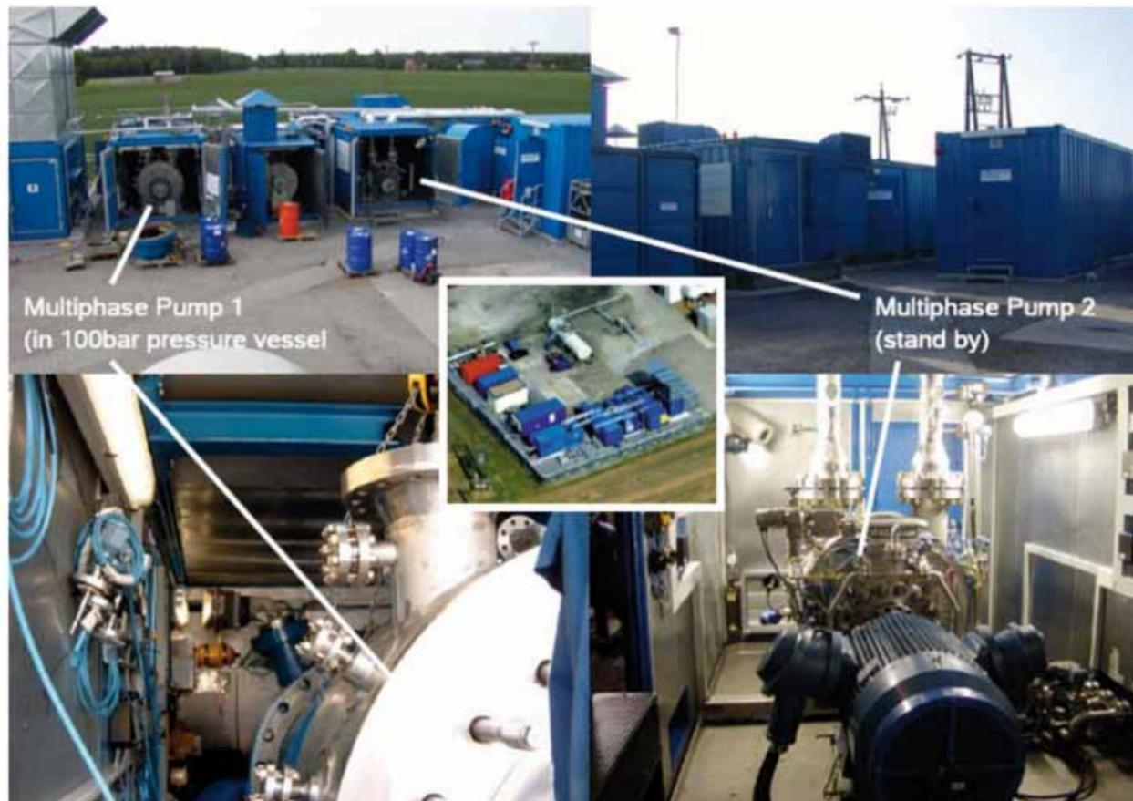
Figure 2: Multiphase test plant Rütenbrock
