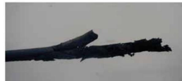
Figure 8: O-ring damaged by explosive decompression
